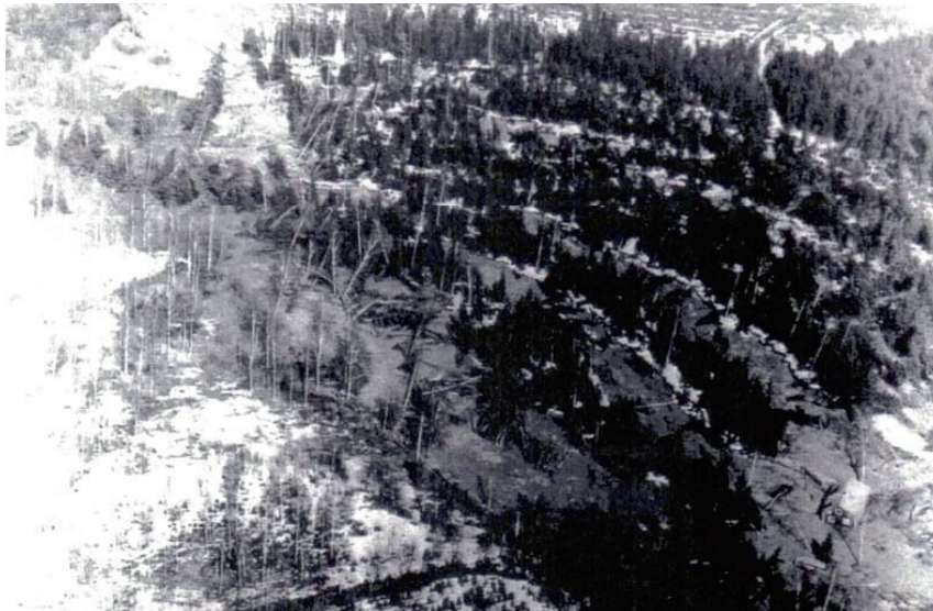
Figure 8:5.1 Aerial photo of the retrogressive landslide along the eastern bank of the Nor River, Sweden.
